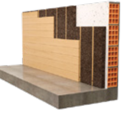
Interior solutions for exterior walls Support for wooden wainscot
