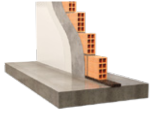
Internal partitions Masonry wall and slab discontinuity
