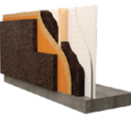
External walls Exterior cladding over wooden substrate - cork at sight
